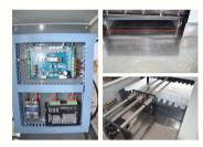
SF-520 series hydraulic and digital paper cutter offers a maximum width of 520mm, capable of handling most commercial paper cutting needs. It is the perfect cutter for print finishing and on-demand working situations.
