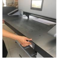
4) When finishing cut, press "PUSH" key to push the papers or books out(if you have set push function it will be done automatically after every cut), then a cut is completed.
