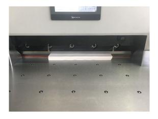
3) After the cut size confirmed and paper put in the right position, downward the foot pedal, clamp the papers, both two hands on the cut buttons to start cutting. Or you don't have to use the foot pedal, only to press the cut buttons with two hands to start the clamp and cut automatically. If you find anything wrong, release the cut bottom to stop the clamp and blade, press only clamp back switch to make the clamp up, make sure everything is right
