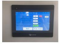
When the paper cut dimension is different from the display dimensions, you can adjust the number to fix it, restart the machine after it is done.
