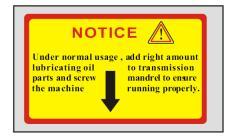
Under normal usage, add right amount lubricating oil to transmission parts and screw mandrel to ensure the machine running properly.
