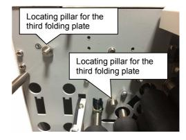
**Note:** The four grooves of the folding plate must be attached to the four Locating pillars completely.
