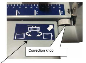
When this case occurred, turn the slant correction knob to correct the misalignment as the guidance showed.
