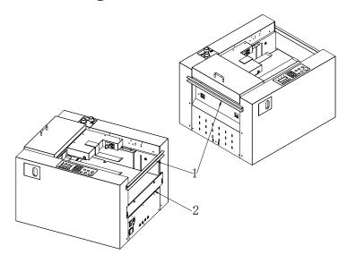
1. Un pack it, install the parts as per above illustration Withdrawing the cover marked 1 and tight the screw, withdrawing the cover marked 2, tight screw the left and right. The two handle screws on the lifting plate are set aside for use.
