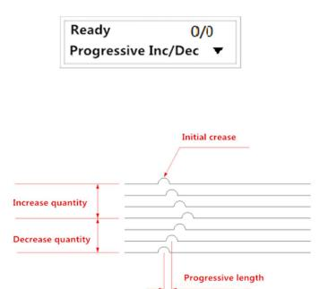
Initial position: the distance from the paper edge to the first crease position, press "enter". Progressive length: increase or decrease based on the Last data. press "enter" button. Increase qty: the increase of paper quantity.
