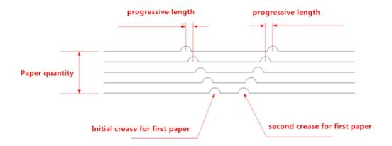
flat back model crease was widely used on wire stiching binding.it is suitable to flat back perfect binding
