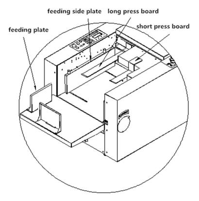
Put the paper into the right place based on the paper size
