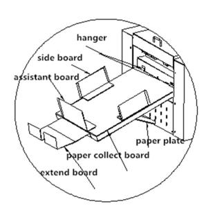
Install the paper collect board in to the two hangers, make sure paper plate lock in to the machine, put the other parts correct same as the photo.make sure all install well before using the machine.
