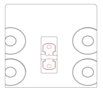
Crease tool install:open the safety cover, put the two crease blade same as the photo shows.
