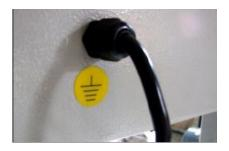
Must use socket with ground wire connected.
