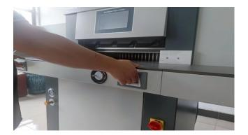
4) When finishing cut, press "PUSH" key to push the papers or books out(if you have set push function it will be done automatically after every cut), then a cut is completed.
