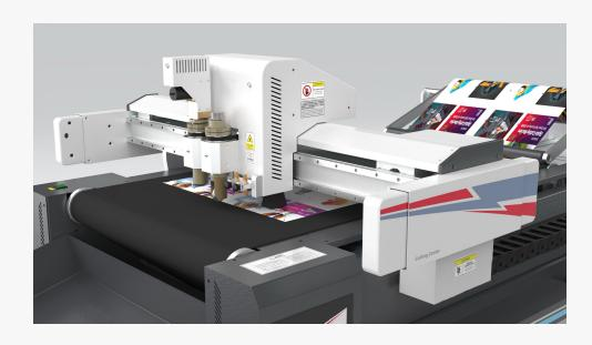
Digital cutting machine model SF-6090 with additional tool module, which makes it possible to use electric oscillating tool, drag tool, V-cut tool, perforating tool on it. CAM software prevents overcut at inner angles to recover graphic outline maximally.
